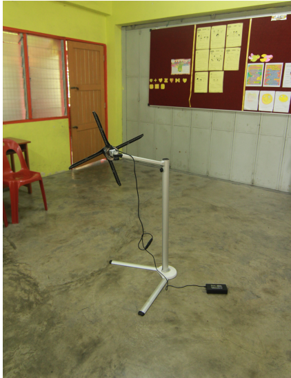
Fig. 1. Fan hologram device used for showing 3D models and animation [6].
