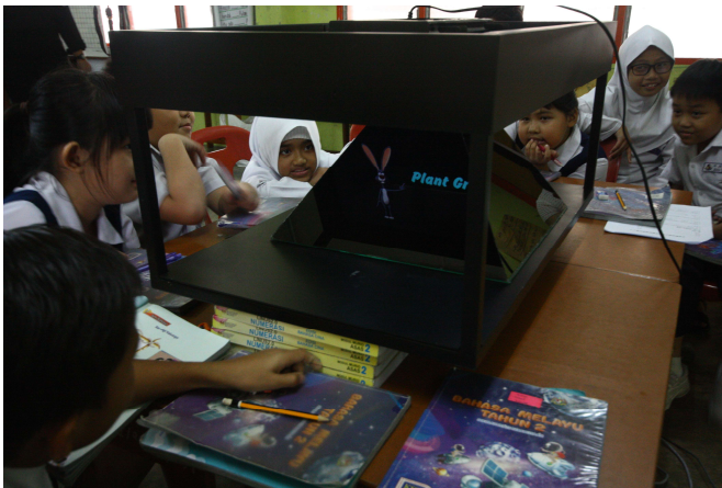
Fig. 2. Pyramid projector hologram device used for showing 3D animation [6].
