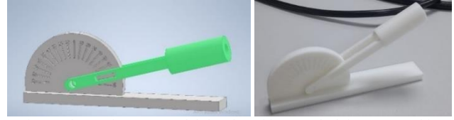
Fig. 4. The goniometer model developed in Autodesk inventor and its product printed using a 3D printer.
